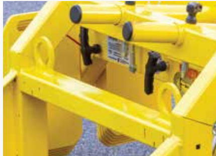
Large Hoisting Rings Built In make the Penetrator 2 +2 easy to lift on to elevated work areas. Perfect for crane use!
