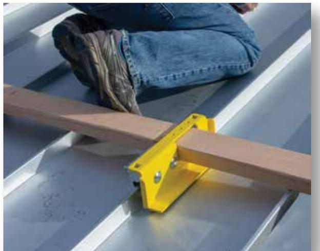
Anchors are Compliant with OSHA 1910 and 1926 Subpart M, ANSI Z359. 1-2007 and ANSI A10.32-2012 Regulations. Specification: 5,000 lbs. minimum breaking strength. Weight capacity: 130-310 lbs.
