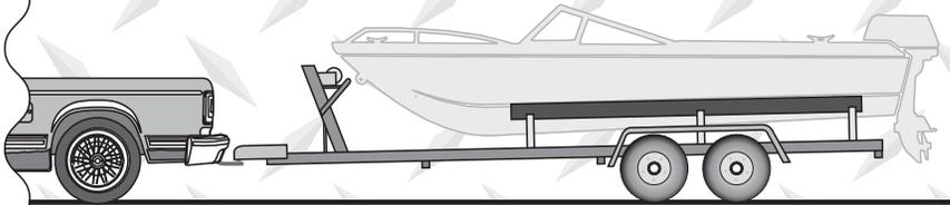
Trailer is not level, note that most of the load is on the front axle
