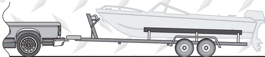
Trailer is not level, note that most of the load is on the rear axle
