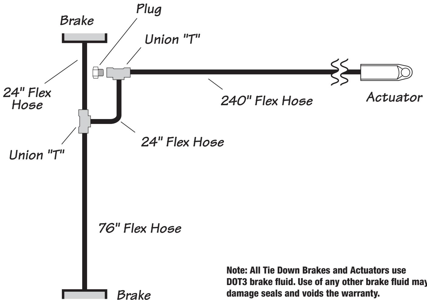
**Note: All Tie Down Brakes and Actuators use DOT3 brake fluid. Use of any other brake fluid may damage seals and voids the warranty.**
